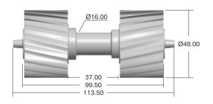
Part no: C 2003 AAH 110 A Autoclean Roller - BTA-E Between Top Arm - End
